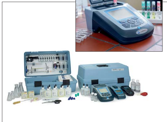
WR840-37/WR840-47 with accessory turbidimeter and pH meter
